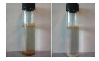
Fig.3: (a) Accumulation of SW at the bottom of vial; (b) MSW remained on the surface of water after 7 days
