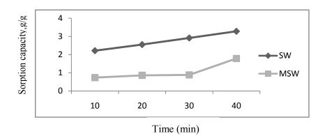
Fig.5: Sorption capacity of SW and MSW in the wet system (static)
