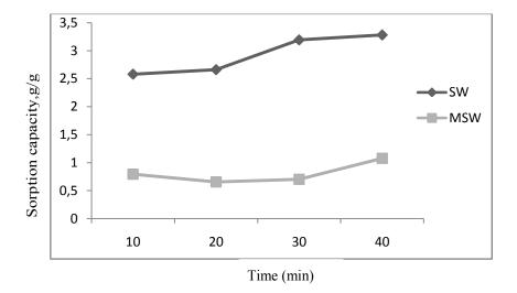
Fig.6: The sorption capacity of SW and MSW in the wet system (dynamic)
